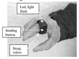
The "Finger Kick" uses the remote as relay for long distance. So it is important that the "Finger Kick" is in the remote's range, i.e. less than 5 metres.
